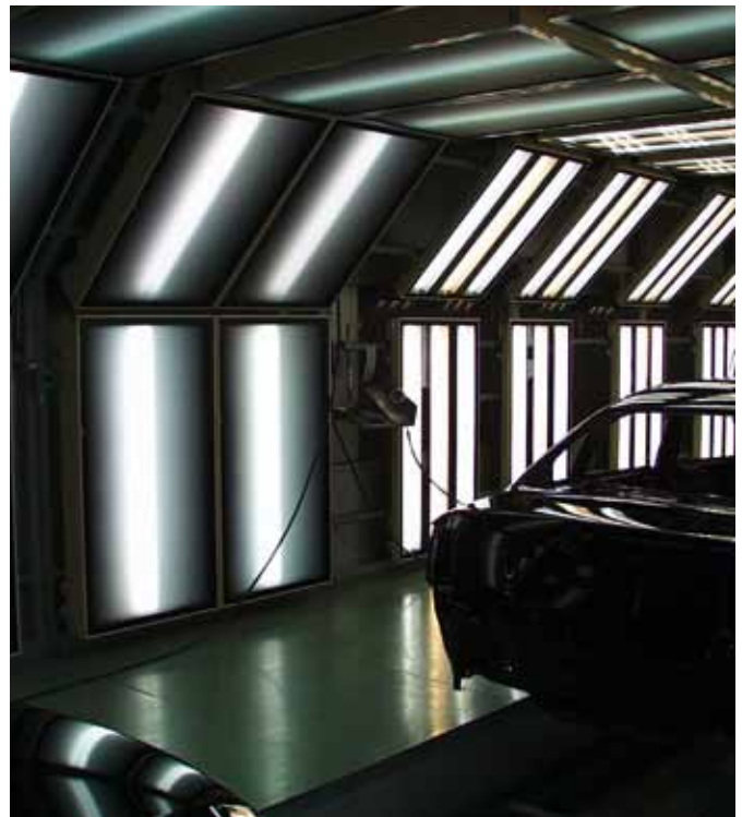
Fig.: Light tunnel in the top coat area
