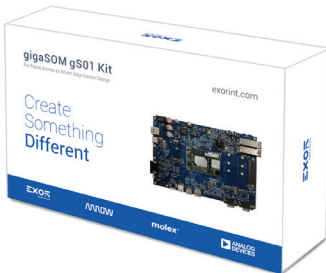
gS01 Development Kit Development Board based on GS01-0004 E3940 plus Cyclone X FPGA Ord. code: +EE16EK-0011
